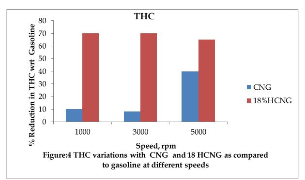
(vi) The THC reduces by 10% with CNG and further reduces by 70% with HCNG even at 1000 rpm compared to gasoline.
